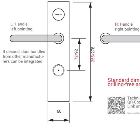
Standard dimensions for drilling-free and simple mounting
